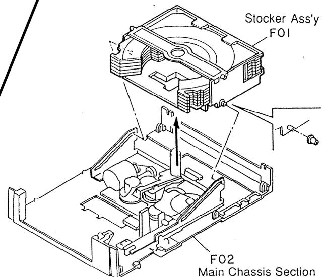
To reinstall tray and stacker: reinstall tray with carriage. Power up and let carriage go in @ disc 1(lowest). Then slide each stacker by hand in to the carriage.
