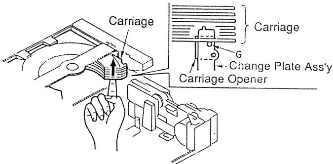
Fig. 2.7.4 Leveling the carriages at the right side
