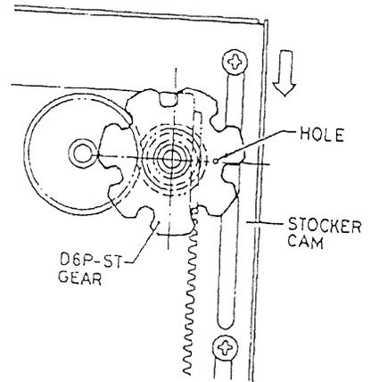
2. Gear positioning in side chassis R section
